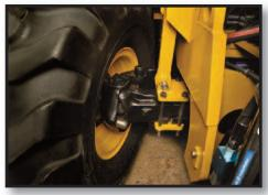
**STEERING CONTROL:** Fully hydraulic power steering with 3 modes (4-wheel, Crab, 2-wheel) provides versatility in the toughest terrains.
