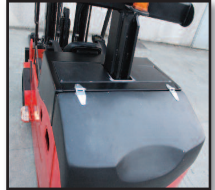
FOPS T-bar roof provides maximum visibility.
