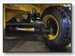
**STEERING CONTROL:** Designed for durability with an extreme duty sandwich type axle. Single cylinder with 4 inch diameter rod, and heavy duty spindles.
