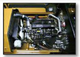
**ENGINE:** The M Series forklifts have a sliding hood for easy access during maintenace, and house a Perkins Turbo Tier 3 emissions compliant diesel engine.
