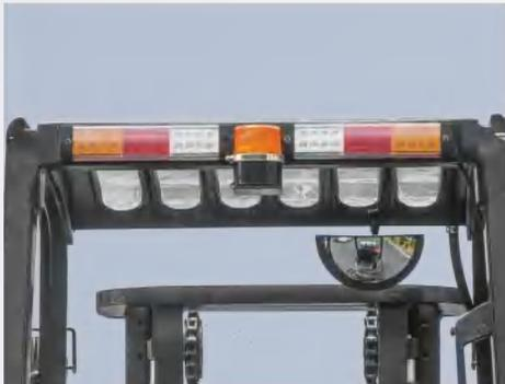
LED lights are applied for entire truck. It saves power and energy, with significantly increased performance and service life of lights.
