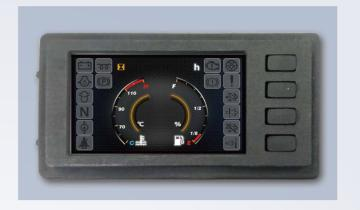
The instrument display is made up of a 4" color LCD screen with four interactive buttons and one CAN bus communication function. The communication protocol is compatible with CANopen and SAE J1939 standards.
