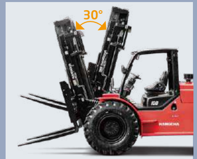
The tilt angle of the mast is 15° in the front/15° in the back, which is more suitable for loading, unloading and transportation of goods in off-road conditions
