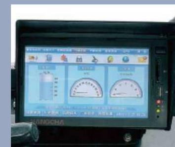
Remote control (optional): Vehicle management system: Vehicle status enquiry and record, alarm for overspeed, door lock, radar and so on. The equipment can be provided with 7-inch touch screen. The operation is simple and convenient. With overall data display & real-time status reminding, monitoring, management and service can be realized in remote way
